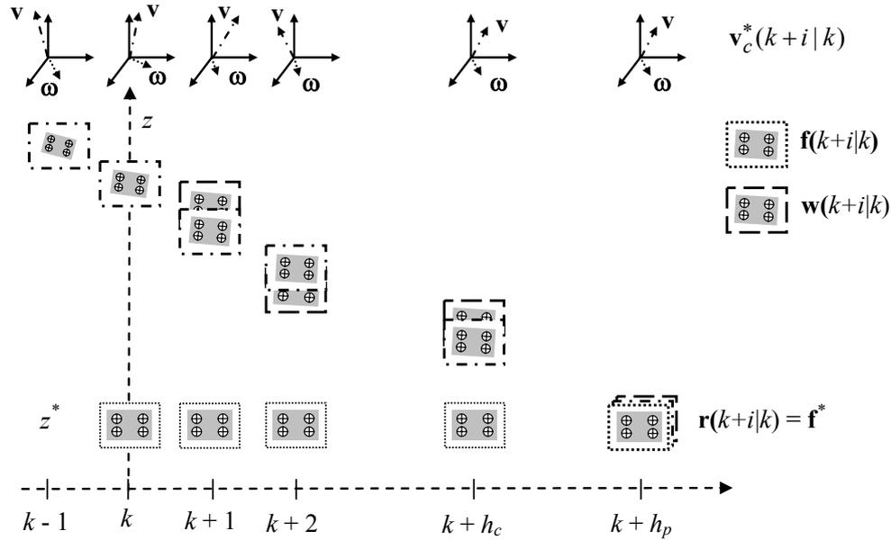
Fig. 2. Predictive control: the basic idea for IBVS applications.
