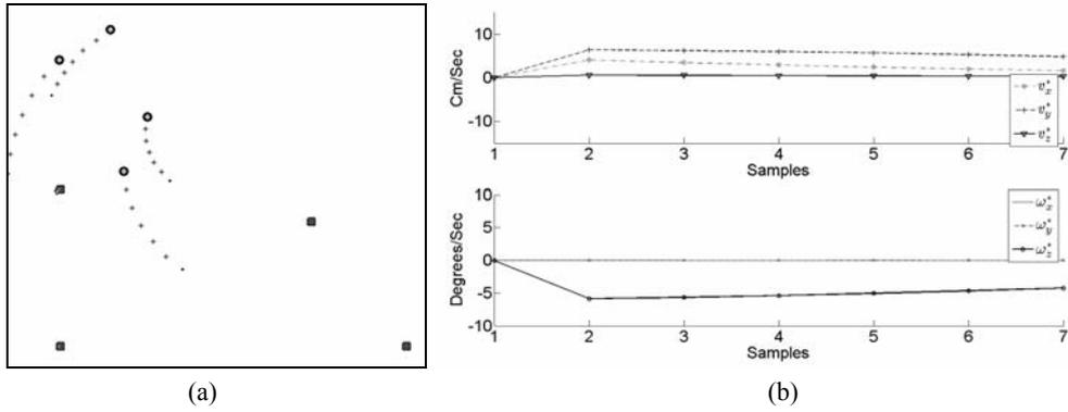
Fig. 4. Proportional controller: a) point features trajectories; b) control effort.
