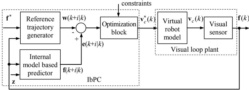
Fig. 3. Cascade structure for robot arm motion predictive control.
