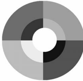
Fig. 2. Iris partitioned in 8 different regions. Color features are extracted for each of these partitions and then concatenated to produce the final feature vector for one iris.
