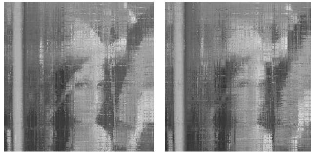
Figure 16 Approximated fuzzy relations obtained by conventional method (left: c = 50 , RMSE = 16.825), (right: c=100 , RMSE = 16.263)
