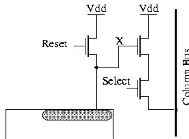
Fig. 2 – CMOS based active pixel sensors
